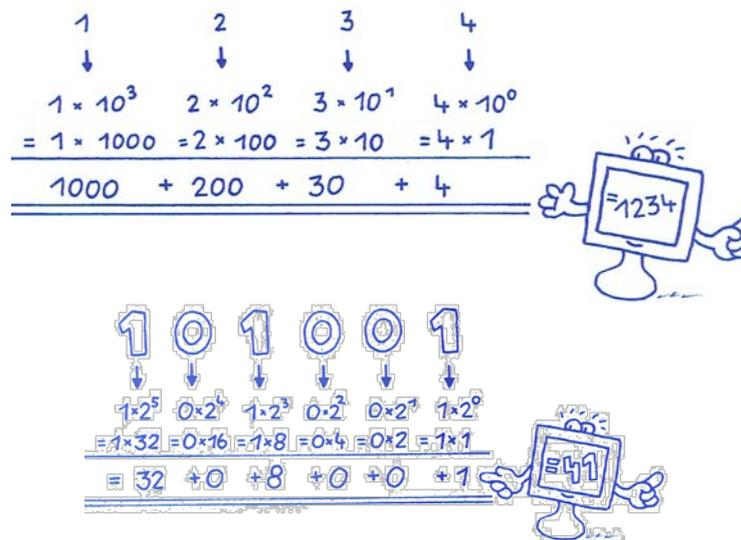
Fig. 2: Examples of decimal (above) and binary numbers [12].
